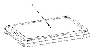
Figure 3.4 Surface cover temperature measurement points
